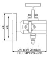
Large-bore Bolted Double Block and Bleed Valves
