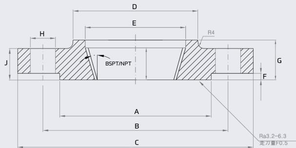
This flange conforms to ANSI/ASME B16.5 and is available in B16/L. Thread is to ISO 7-1
