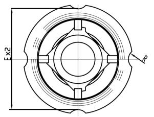
NERO's range of Wafer Disc check valves are made from all 316 material and have a metal to metal sealing face. They are designed to fit between our whole range of flanges as listed below:
