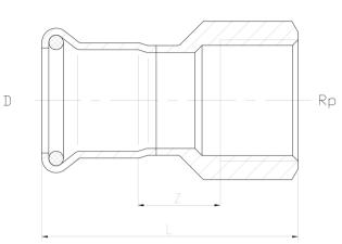
GDPRESS fittings offer reliable and consistent performance, combined with an easy installation process using common M-countour design and tooling compatability.
