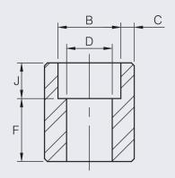
NERO's range of Half Couplings are available in BSPT, BSPP, NPT and Socket Weld configurations
